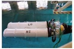
The UK's dependence on energy from non-renewable sources is being challenged by a new wave energy converter called Anaconda that mimics the action of a sea snake. Now in final proof of concept testing at QinetiQ's facilities, Anaconda is producing energy data at an estimated cost that is excitingly low and as such may offer a serious and cost effective alternative in the delivery of future clean energy supplies.
