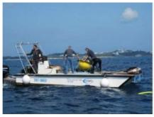
Carnegie Wave Energy(Australia) and its Bermuda-based developer Triton Renewable Energy have successfully deployed and commissioned a wave monitoring buoy off the south shore of Bermuda. This buoy is to gather data to quantify the wave energy resource in support of a potential CETO wave energy project in Bermuda.
