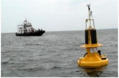
Axys Technologies sees a demand for its buoys, resulting in deliveries all over the world. The Marine Institute at Memorial University in Newfoundland has recently deployed two new monitoring platforms into their SmartBay monitoring network. A 3 metre aluminum discus buoy and a 1.75 Metre WatchKeeper buoy recently dropped anchor into two locations on Placentia Bay (Come by Chance Point and the Pilot Boarding Station).
