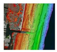
Woolpert has been granted a patent by the United States Patent and Trademark Office for its 'Airborne Topo-Bathy Lidar System and Methods Thereof'. A Lidar sensor system was developed by a multidisciplinary research and development team incorporating these technologies that enable the collection of high-resolution
