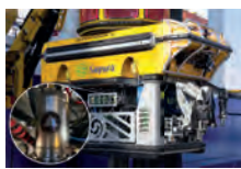
▲ Sapura ROV equipped with an Exail Rovins Nano INS.
