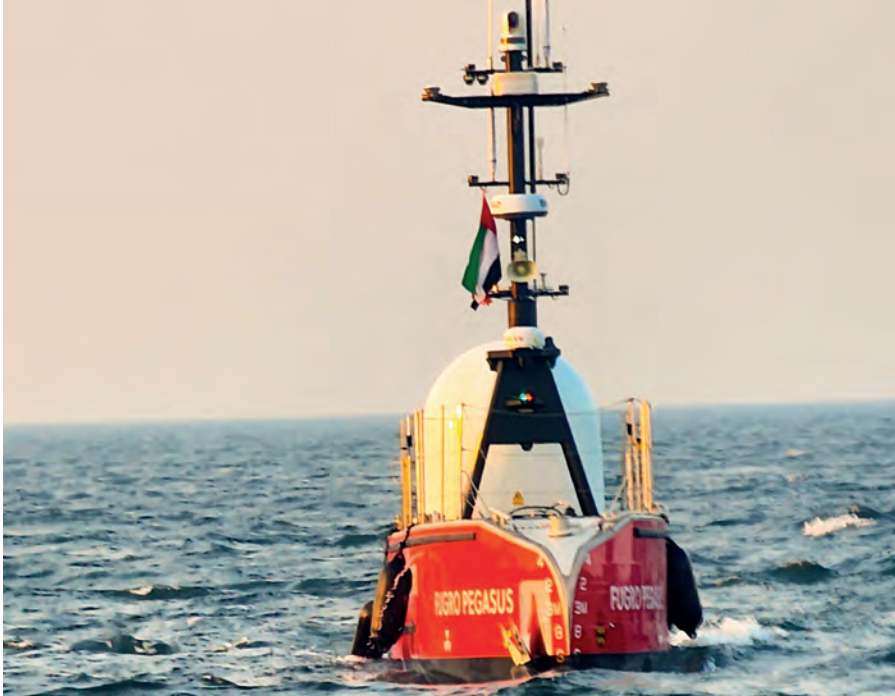
▲ The Fugro Blue Essence USV in the North Sea, built by partner SEA-KIT.
