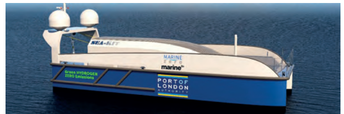
▲ ZEPHR, the Zero Emissions Ports Hydrogen Refilling Survey Vessel. (Image courtesy: SEA-KIT International)
