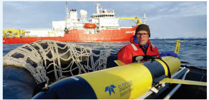
▲ Teledyne Slocum gliders, which are capable of moving at various depths throughout the water column, have become indispensable tools for monitoring ice melting beneath Antarctic ice shelves.
