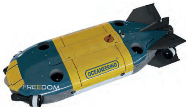
▲ The Freedom AUV/ROV is designed for long-term, deepwater surveys.
