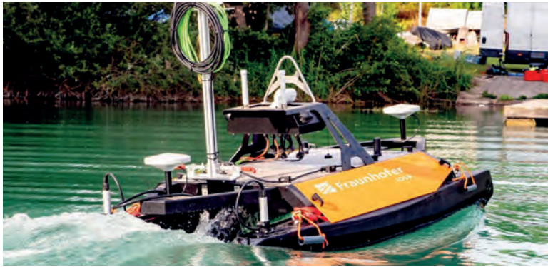
▲ The USV, furnished with autonomous capabilities and an array of sensors for both surface and underwater mapping, is actively engaged in the TAPS project. (Image courtesy: Fraunhofer IOSB)
