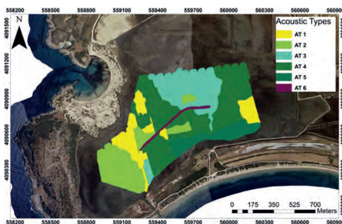
▲ Figure 7. Map showing the lagoon floor acoustic types (AT), as defined by the manual classification based on the sidescan sonar mosaic and the unsupervised classification (SonarClass).
