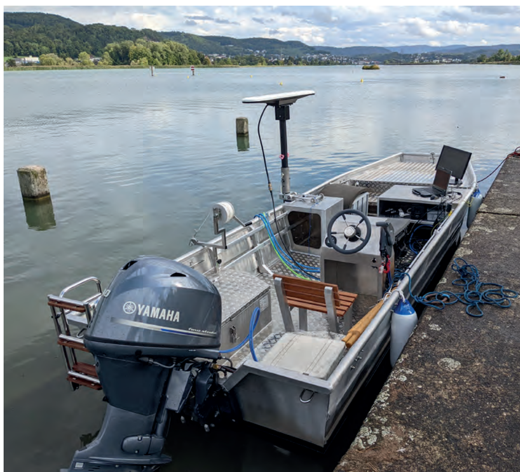
▲ Figure 1a & 1b: Axpo's new survey boat is small, but importantly features a flat bottom for solid seakeeping and a rigid mount for the installation of the bathymetric sonar and its components.
