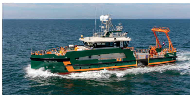
▲ Figure 2: Built by the Royal Niestern Sander shipyard, the Geo Ranger is a support vessel specifically designed for shallow water surveys and serves as the flagship of Geo Plus . The vessel was carefully crafted with both the crew and survey equipment in mind, while placing special emphasis on sustainability. (Image courtesy: Royal Niestern Sander)
