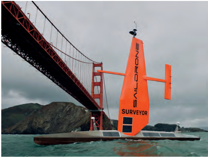
▲ Figure 3: Saildrone's fleet of small and medium-sized USVs offer high-quality bathymetry solutions for both near-shore and open-ocean applications that meet, and even surpass, the rigorous standards set by the IHO. (Image courtesy: Saildrone)
