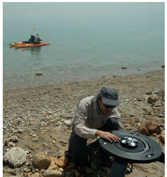
▲ The shore of the Dead Sea is covered in gravels and other sediments of different sizes. Using the Signature1000 ADCP, the researchers unpacked the role of the wave climate in longshore sediment sorting. (Photo: Nadav Lensky)
