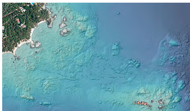
▲ Figure 2: This image depicts the region surrounding the Formigues Islands, situated in the northern region of Catalonia. The bathymetric depth model provides complete coverage of the area, with the darkest blue hue indicating depths exceeding 30 meters.
