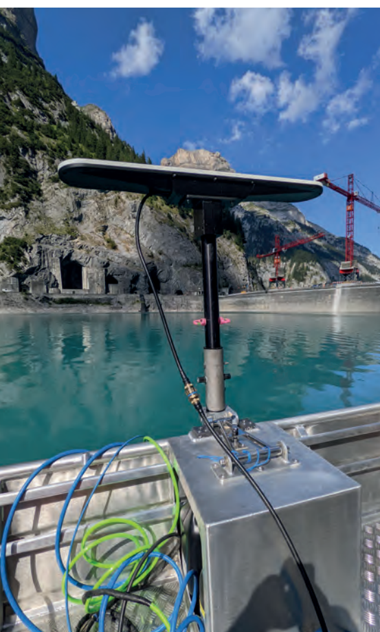
▲ Figure 1a & 1b: Axpo's new survey boat is small, but importantly features a flat bottom for solid seakeeping and a rigid mount for the installation of the bathymetric sonar and its components.
