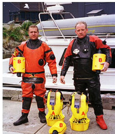
Figure 2: A dive team (Envirotech Diving) with their AquaMap LBL acoustic underwater positioning system including three baseline transponders (B) and diver stations (A) mounted on scooters. The baseline stations are first deployed in the corners of a work site. Their relative position is then precisely measured using the AquaMap system's automatic acoustic self-survey capability. For geo-referenced operations, the baseline positions are surveyed by differential GPS or a laser positioning equipment (total station). During a dive, the diver station interrogates the baseline stations to measure the distances, which are then converted to positions.
