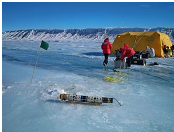
Figure 2: The SCINI ROV next to its dive hole at Heald Island, Antarctica
