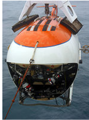
Figure 3: The Russian deep sea submersibles MIR-1 and MIR-2 searched the wreck site of the Japanese submarine I-52 in 1998. A LBL positioning system was used to guide and document the progressing search over multiple dives.
