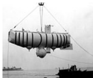
Figure 2b: The bathyscaphe Trieste was guided by that acoustic positioning system to the Thresher
