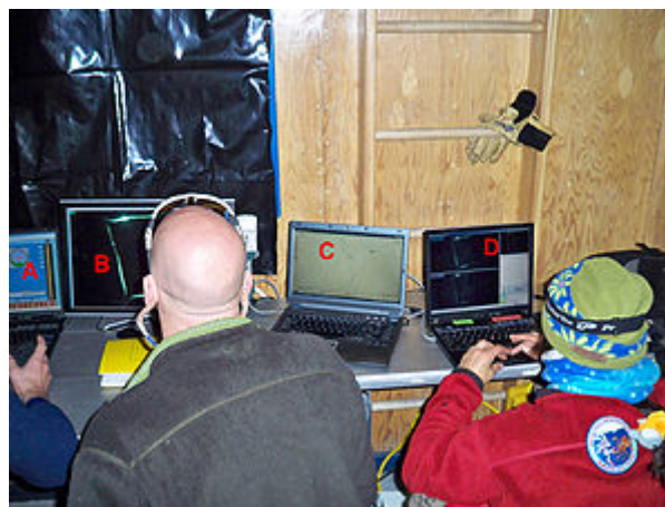
Figure 4A: SCINI control room with four display screens for ROV control (A), main camera view (B), SBL navigation display (C) and image annotation or science screen (D)
