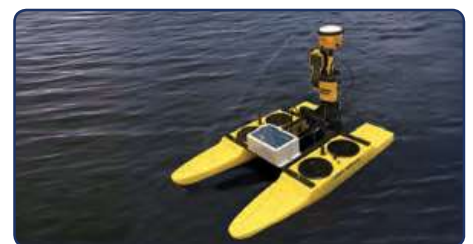
HyDrone™ ASV with Trimble SPS 585 and TSC3
