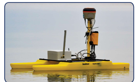
HydroLite-TM™ with Trimble GPS and data collector
