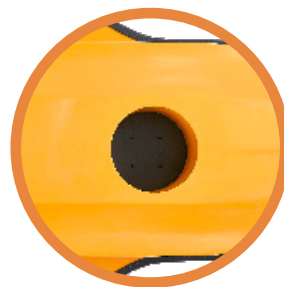
ADCP access shaft
