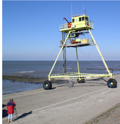
Figure 1: The WESP being measured using photogrammetry (picture by A.P.M. Pieters)
