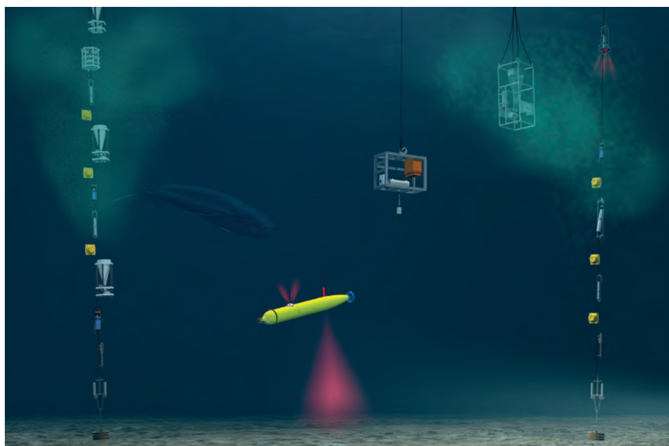
▲ Figure 3: Moorings with instruments and an AUV used by the Alfred Wegener Institute. (Courtesy: AWI, Bremerhaven/FRAM/Sabine Lüdeling)
