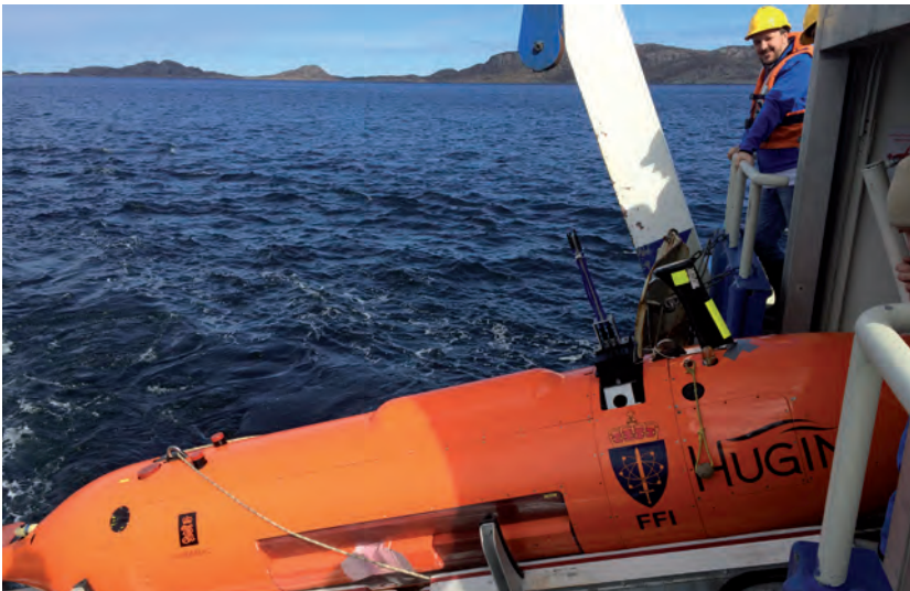
▲ The HUGIN AUV collected bathymetric data and identified pre-set targets.
