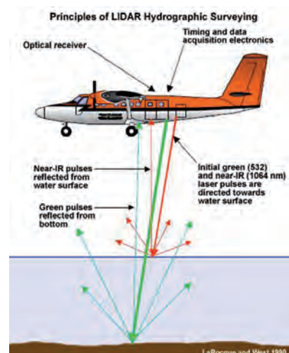
▲ Figure 3: Principles of Lidar hydrographic surveying. (Source: LaRocque and West)
